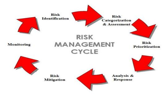
Risk Management cycle can be broken down in two broad sections with first focusing on the identification, categorisation and prioritisation of risk. The second section focuses on the mitigation and monitoring of the risks. The diagram below represents the main activities undertaken in the two broad sections:
